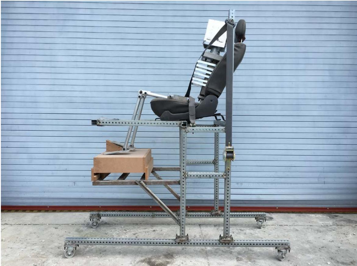
**Figure 3.16** Simplified dummy and sled rig
