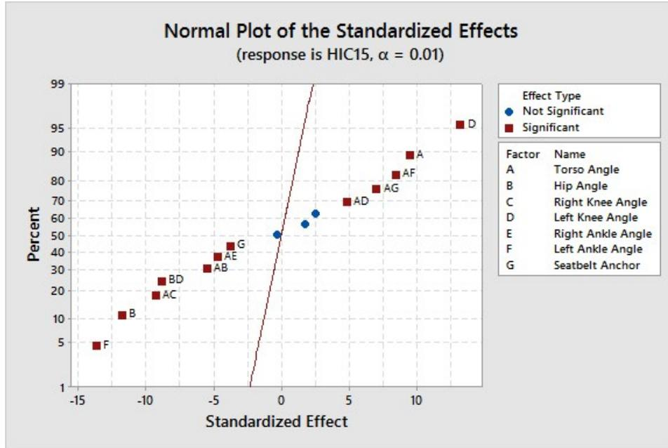
Figure 4.12 Significant factor plot for  $HIC_{15}$
