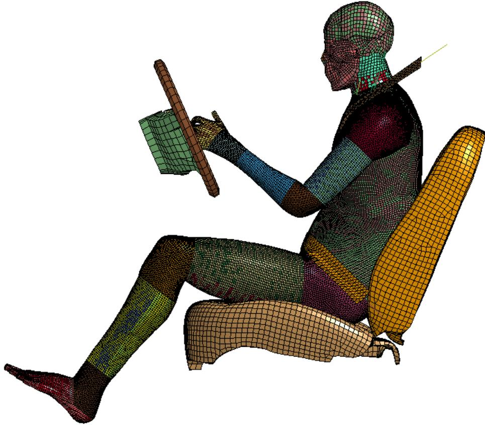
**Figure 3.7** THUMS Simulation Setup with Steering Wheel and Airbag
