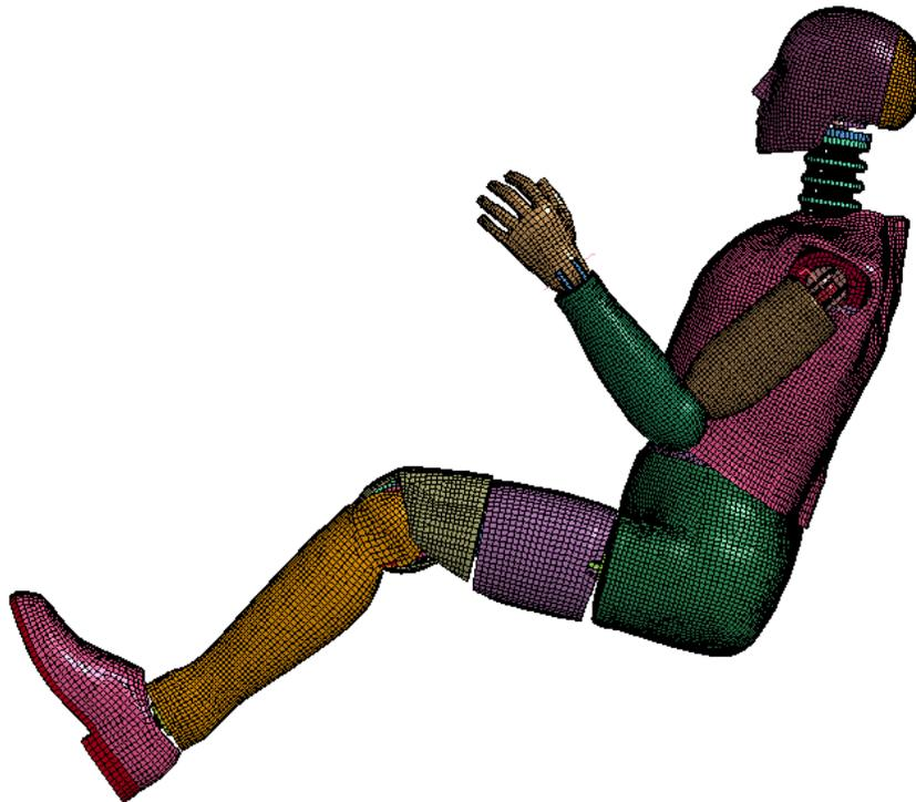
**Figure 3.3** Hybrid III 50<sup>th</sup> percentile dummy model
